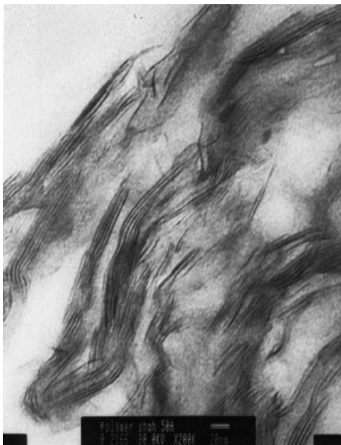
Figure 1. TEM image of a 5.0 wt % CLO (3.05 wt % MMT) nanocomposite sample at 200,000 \times magnification.
