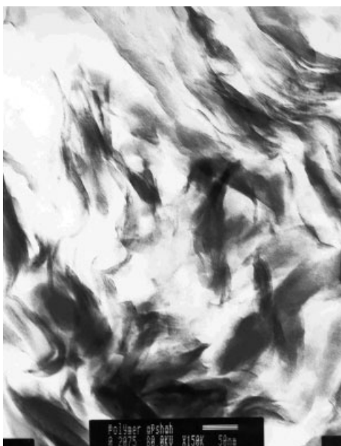
Figure 2. TEM image of a 5.0 wt % VMC (3.9 wt % MMT) nanocomposite sample at 150,000 \times magnification.
